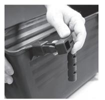
Turn the "A" arm so the "A" is facing toward the Fuel Tank.
